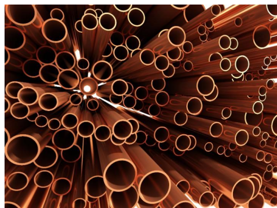
C106: readily welded and brazed for tubes
